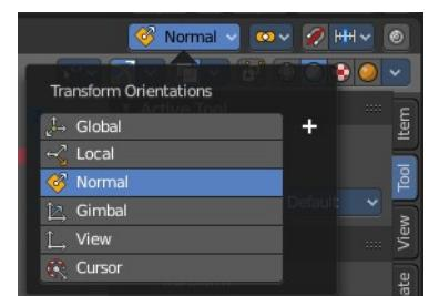
By holding down the mouse button and pressing the X, Y or Z key twice you can toggle this to local. But also to other orientations. This depends in what orientation you start. With normal you can toggle that way between Normal and Global.
