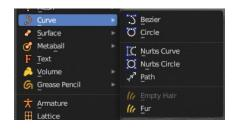
Curve objects are mathematical curves that are defined by a start and endpoint. You can edit the shape of the curve by handlers. Curves have several purposes. They can be used as a path. Or you use them as the base for a mesh object.
