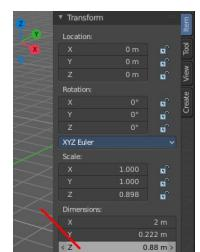
In the header you can see the height of the extrusion. In the Transform panel in the sidebar you can adjust this height also afterwards. The Z value.
