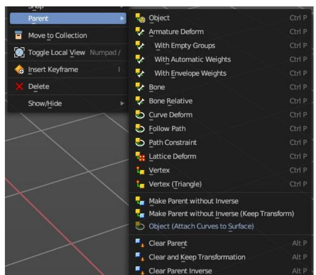
The methods are object type dependent. The armature methods requires to have a mesh and an armature. The path methods a curve. The available methods for the current selection can also be found out by pressing the hotkey ctrl P. This calls the parenting menu with just the available methods.
