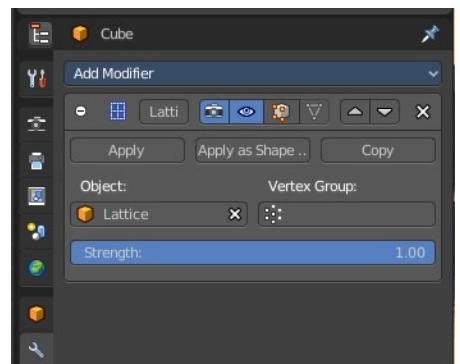
Take care of the position and size of the lattice object. It influences how the deformation works.
