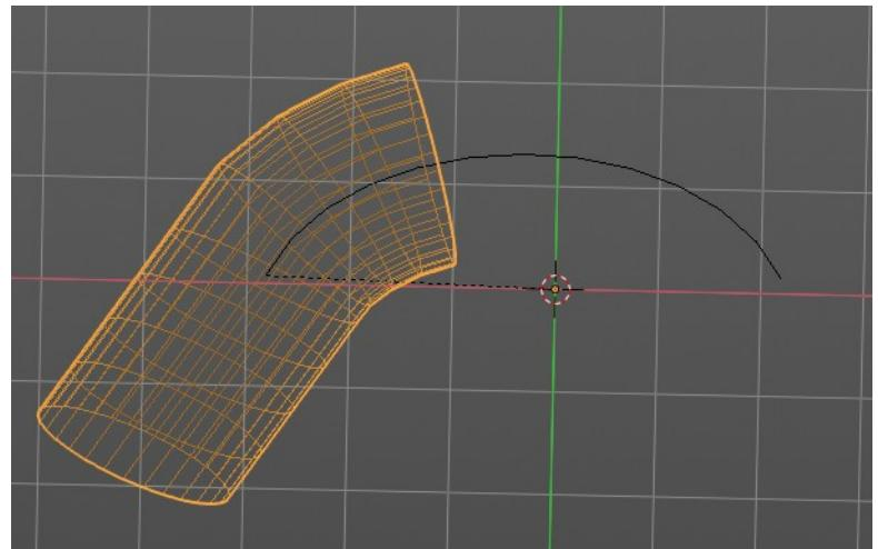
To demonstrate the only pitfall, by parenting the center of the object goes to the start point of the curve. So you better put the origin at the bottom of the cylinder before parenting.
