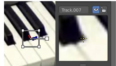
If an anchor is used (the position in the image which is tracking is different from the position which is used for parenting), a preview widget will display the area around the anchor position.
