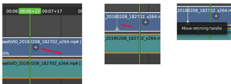
The retiming happens from marker to marker per section. The new playspeed of the marker section can be seen at the clip then.
