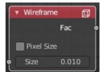
Meshes are triangulated before being processed by Cycles. So the topology will always appear triangulated when viewed with the Wire frame node.
