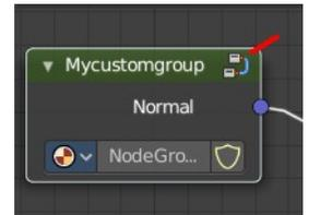
A group can be further collapsed by clicking at the triangle button in the upper left corner.
