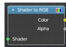
The Shader to RGB node is typically used for non-photo realistic rendering, to apply additional effects on the output of BSDFs. For example, a color ramp on the output of a diffuse BSDF can be used to create a flexible toon shader.
