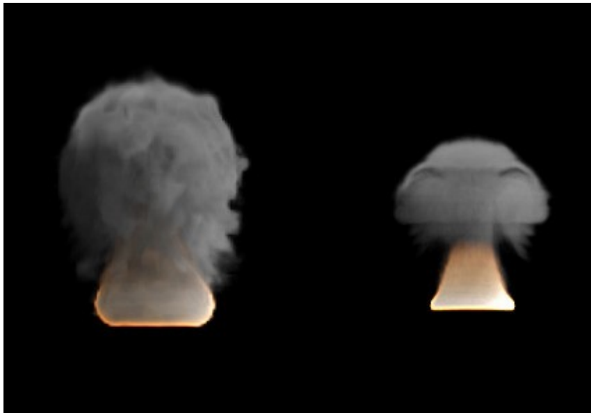
Comparison between a domain with 24 divisions and 4 High Resolution divisions (left), and a domain with 100 divisions and 1 High Resolution division (right).
