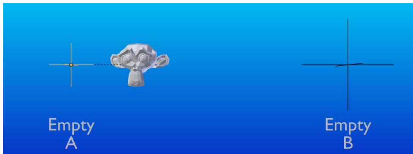
Figure 2 - Scene with Monkey object being the Child Object of “EmptyA”. “EmptyA” has been scaled resulting in the Monkey also being scaled and moved to the left.
