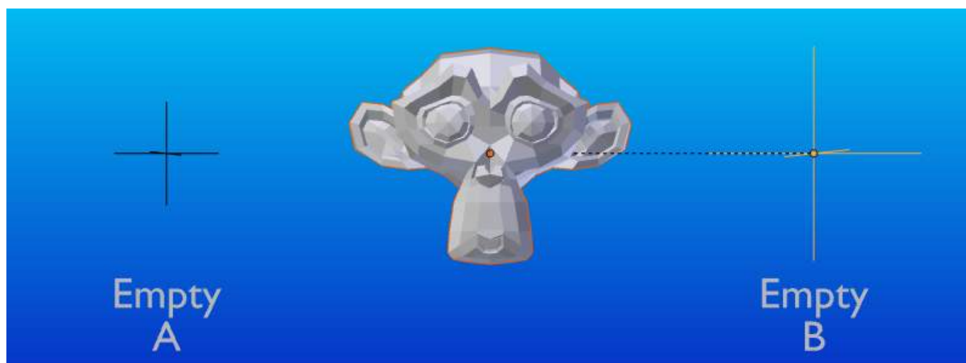
Figure 3 - Scene with Monkey object having its a parent changed from “EmptyA” to “EmptyB” and the resulting change in scale.
