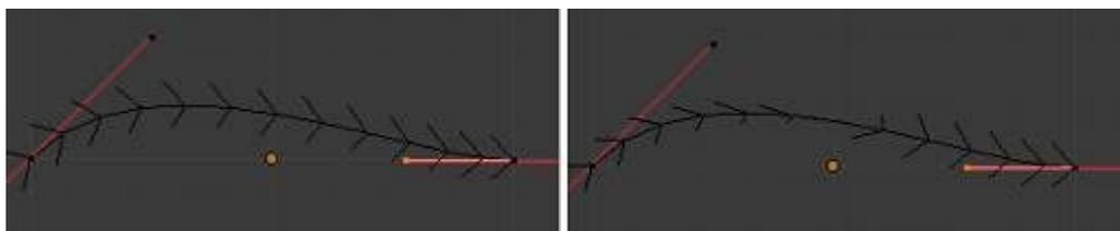
Curves with a twist of minimum (left) and tangent (right).
