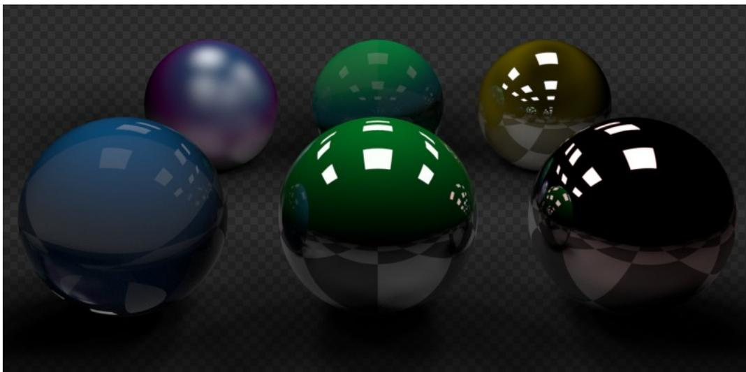
Example of the shadow catcher. Note how the material of the plane can still be viewed in the spheres.
